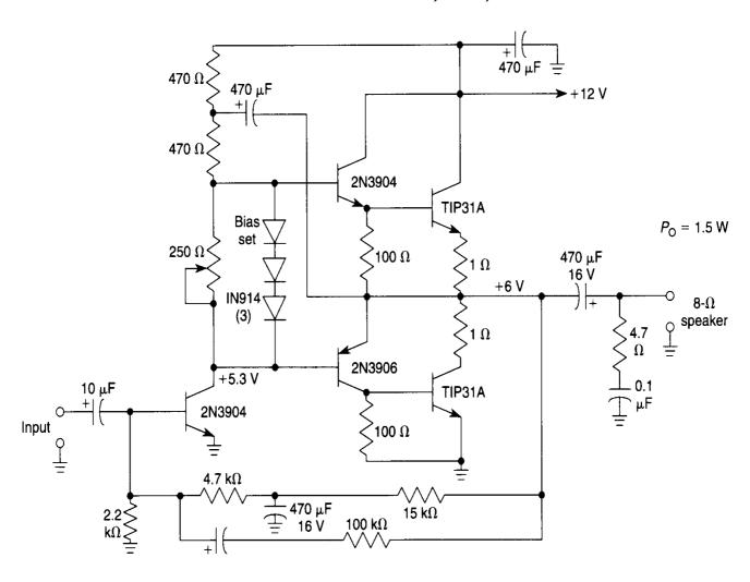
Although ICs have largely replaced circuits such as this, this circuit still finds use where the flexibility of a discrete device design is desirable. Parts are easy to obtain and the problem of IC obsolescence is eliminated. The TIP31A can be heatsinked to a small metal heatsink, if desired.
